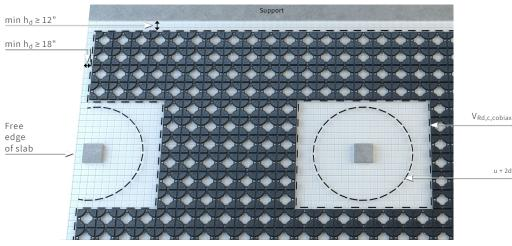
Approx. 50% to 80% of the slab area is fitted with void formers (may vary according to different structural configuration
